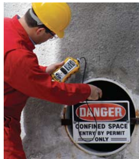
Confined space testing with the MultiRAE Lite
