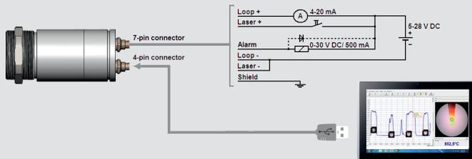
Analog operation mode: 4-20 mA and alarm interface. Setup & installation via USB cable (hot Plug & Play)
