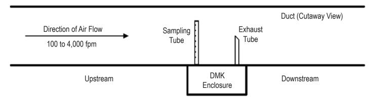
Sampling and exhaust tubes must be installed in the proper orientation to ensure good air flow through the DMK-1 and to the gas detector
