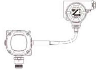
Remotely mounted sensor
