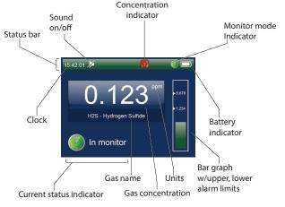
Figure 3: SPM Flex display - In Monitor mode
