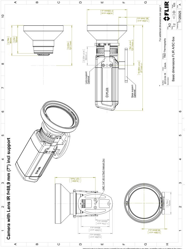
© 2012, FLIR Systems, Inc. All rights reserved worldwide. No part of this drawing may be reproduced, stored in a retrieval system, or transmitted in any for by any means, electronic, mechanical, photocopying, recording, or otherwise, without written permission from FLIR Systems, Inc. Specifications subject to change without further notice. Dimensional data is based on nominal values. Products may be subject to regional market considerations. License procedures may apply.
