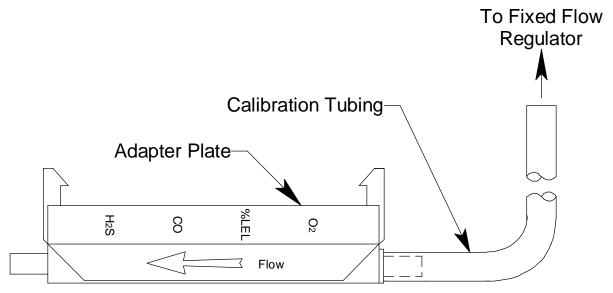
Figure 26: Calibration Kit Assembly
