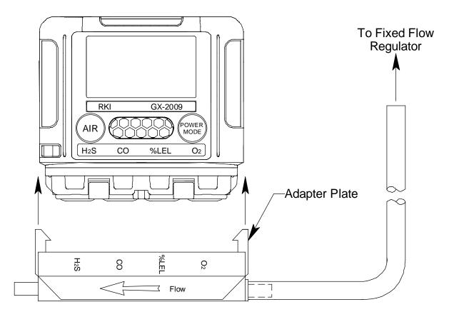
Figure 27: Installing the Adapter Plate, Auto Cal
