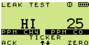
Fig. 12.4 HI LEL Alarm
