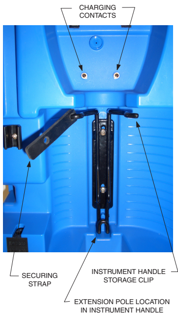
Fig 13.20 Charging Station - Instrument Location
