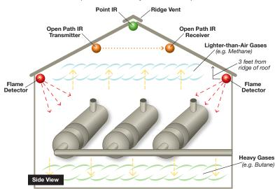
Effective monitoring of compressor facility could include flame detection, point infrared hydrocarbon gas monitoring, or a mix, depending on variables unique to each site.
