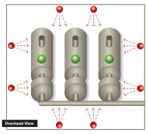
Blanket protection of engine area, shown here, includes perimeter monitoring with flame detection, and flammable gas detectors placed over the equipment to monitor flammable gas that has a tendency to rise because of its lighter-than-air density and weight (e.g. methane).
