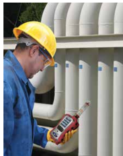
MultiRAE Benzene used for leak detection
