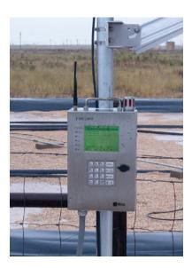
The FMC-2000 controller can monitor up to 24 wireless MeshGuard detectors and contains five programmable relays that can trigger external alarms or process controls.
