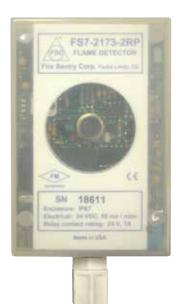
The Fire Sentry FS7-2173 electro-optical radiant energy fire detector and the Fire Sentry FS7-2173-2RP (unitised model) with multi-spectral WideBand IR™, Near Band IR and Visible Band fire detection are designed specifically for semiconductor clean room fire protection applications. The FS-2173-2RP is standalone and FS-2173 interfaces to a control module.
